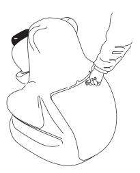
**5** Simply push door panel back into its original position and lock turning clockwise with special key provided.
