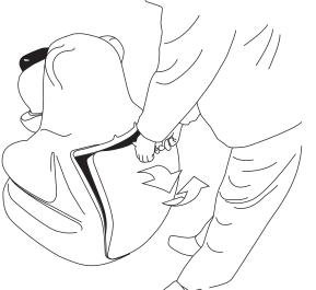
1 Using the key provided, turning anti-clockwise, unlock and pull the door away from the main body. The door can then be lifted off and placed to rest.
