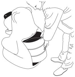
2 Lift and slide out the galvanised steel liner using the two drop handles provided.
